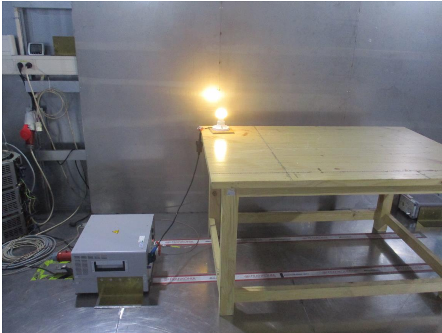
Photograph 1: Set-up for measurement of conducted emission
