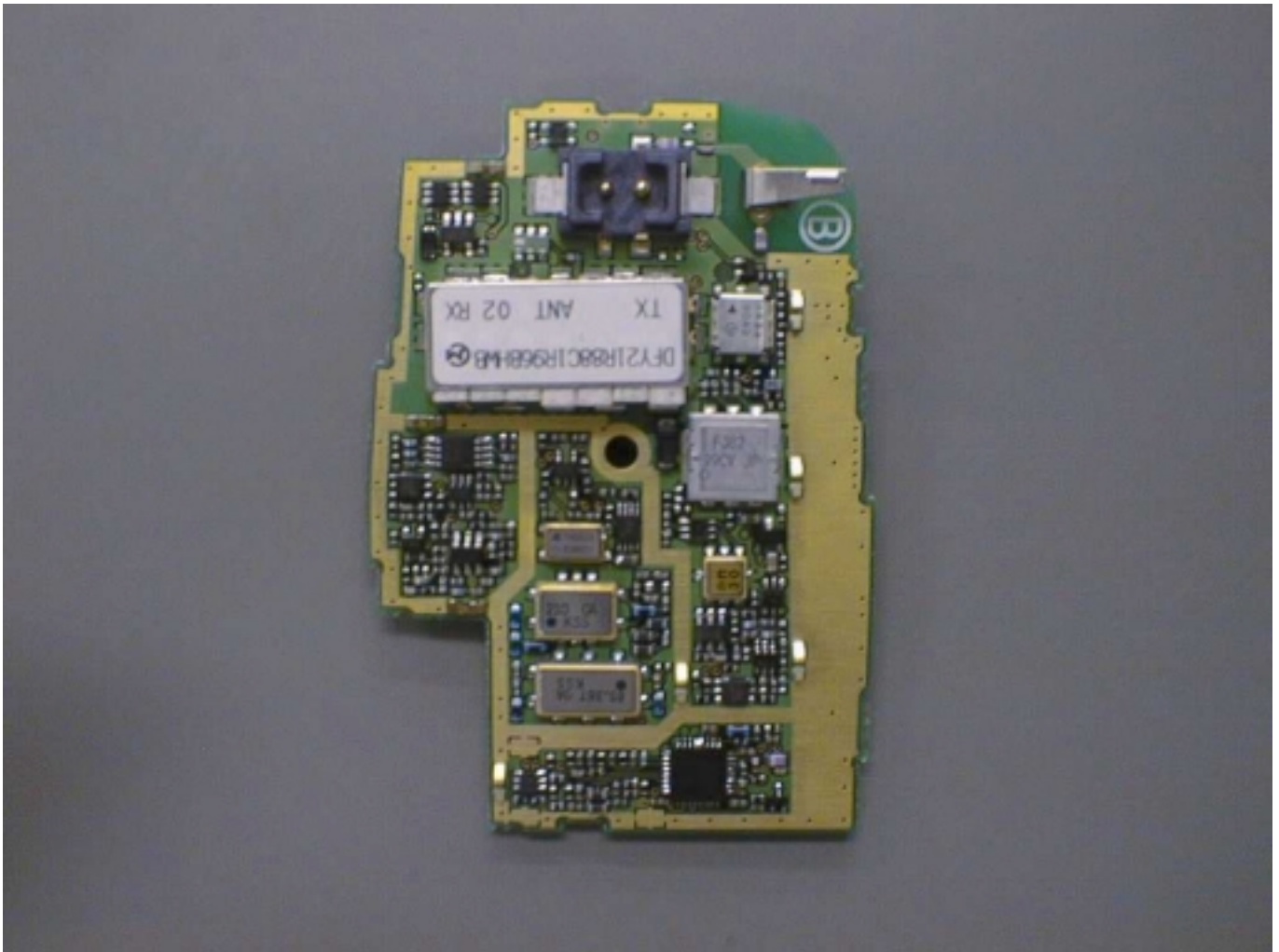
Handheld Portable TR Board (With Shelled Cover Removed) (VC-TCXO: KT18-ECW27A-19.680MT)
