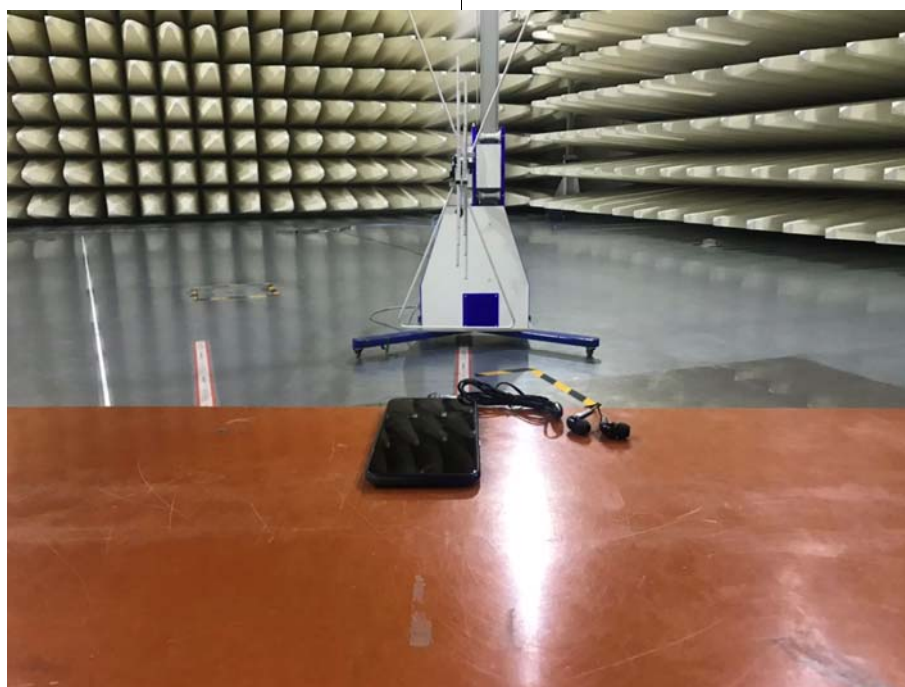
Radiated Emissions Test Setup (with charger) (30-1000MHz)
