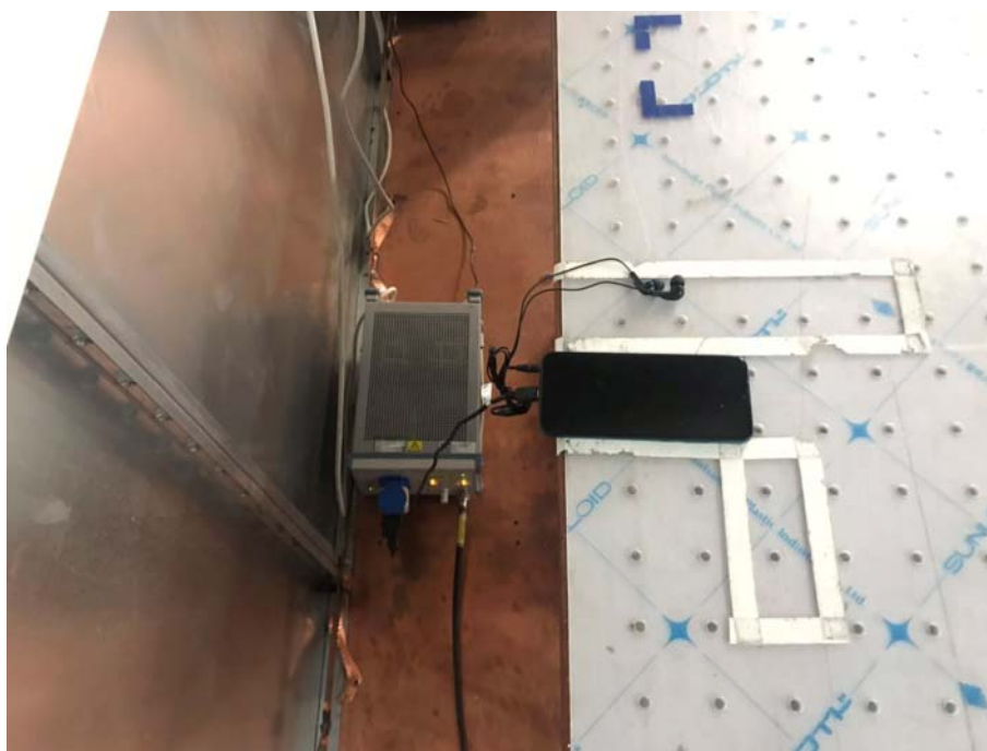
Conducted Emissions Test Setup (with charger)
