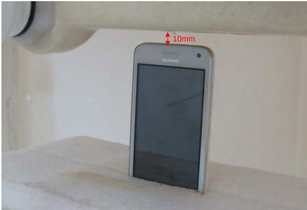
Picture 17: Top Edge, the distance from handset to the bottom of the Phantom is 10mm
