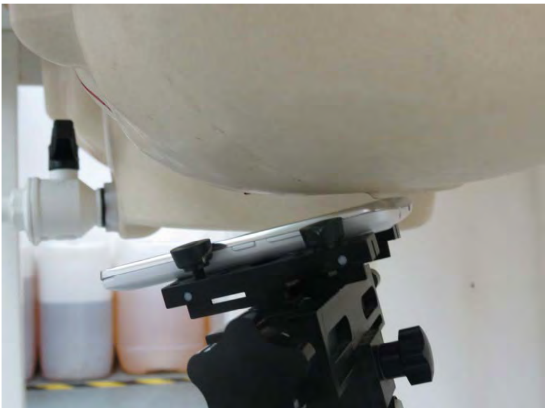
Picture 10: Left Hand Tilt 15 Degree Position
