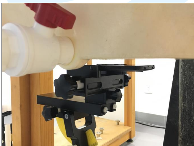
Front Face of EUT with 1.0 cm Gap
