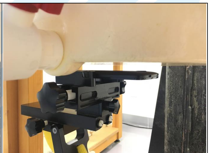
Rear Face of EUT with 1.0 cm Gap
