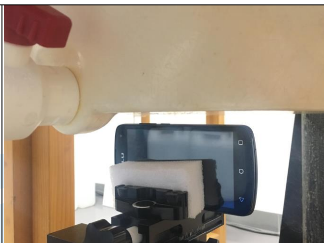
Right Side of EUT with 1.0 cm Gap
