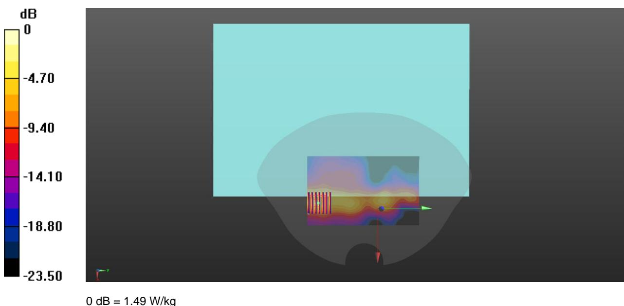
**MEAS.3 Body Plane with Bottom Side 0mm on Middle Channel in 802.11b mode with Antenna Main**
