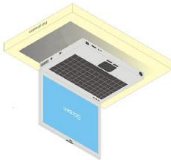
Note: For feet in Laptop, the antenna location can be positioned against the user during normal use and the additional separation introduced by such protrusions between the outer housing and a flat phantom is <5mm;
