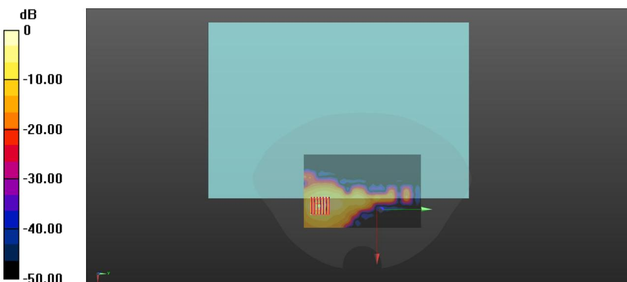
**Meas.9 Body Plane with Bottom Side 0mm on 155 Channel in 802.11ac80 mode with Antenna Main**
