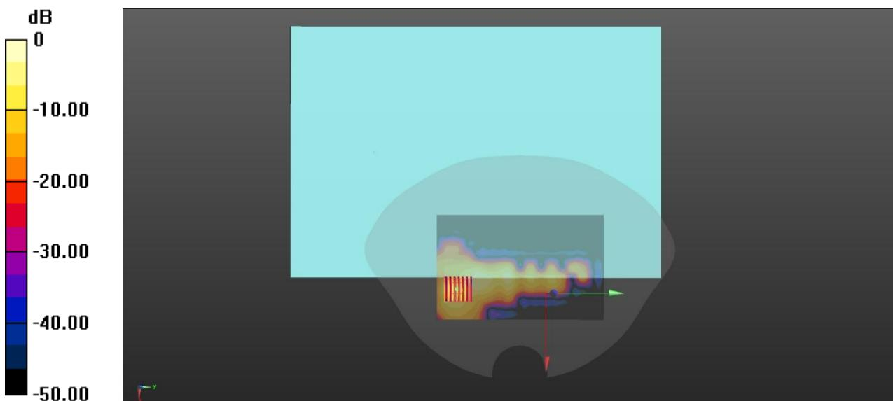
**Meas.5 Body Plane with Bottom Side 0mm on 58 Channel in 802.11ac80 mode with Antenna Main**
