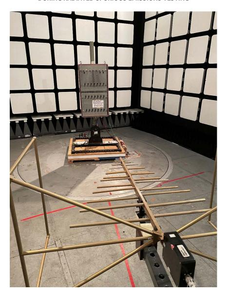
PHOTOGRAPH(S) OF EUT ARRANGEMENT DURING RADIATED SPURIOUS EMISSIONS TESTING
