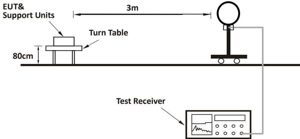
For Radiated emission 30MHz to 1GHz:
