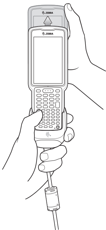
Figure 118 Disconnecting the USB Charge Cable
