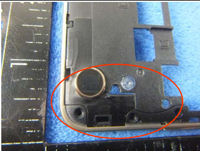
LTE - Antenna View
