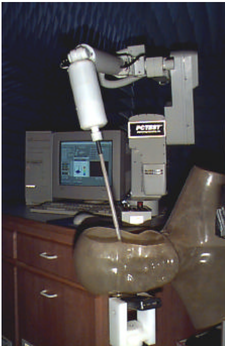
Figure 5. Photograph of the Probe and the Phantom
