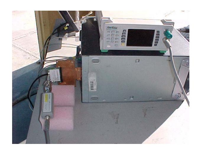
Maximum Peak Output Power Measurement Setup
