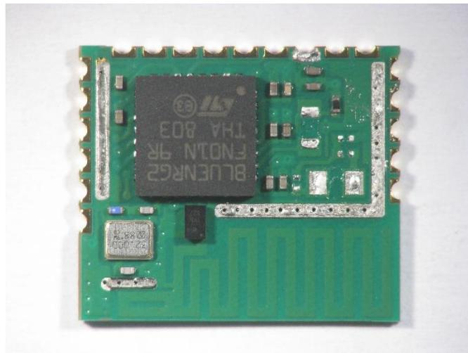
Photograph showing a BLUENRG-M2SP, with shield removed.
