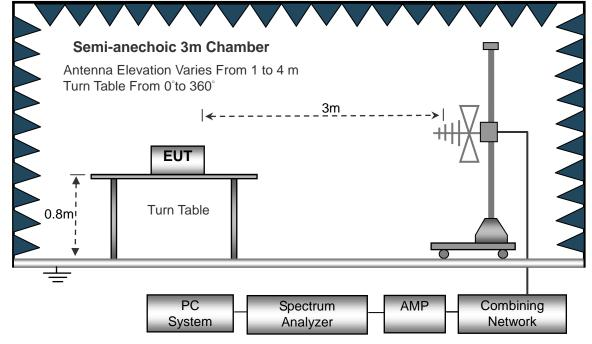
(C) Radiated Emission Test-Up Frequency Above 1GHz
