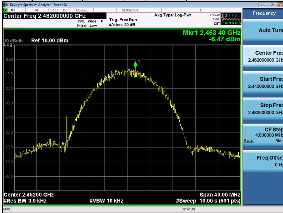
**Power Spectral Density, 2462 MHz, Non HT20, 6 to 54 Mbps**
