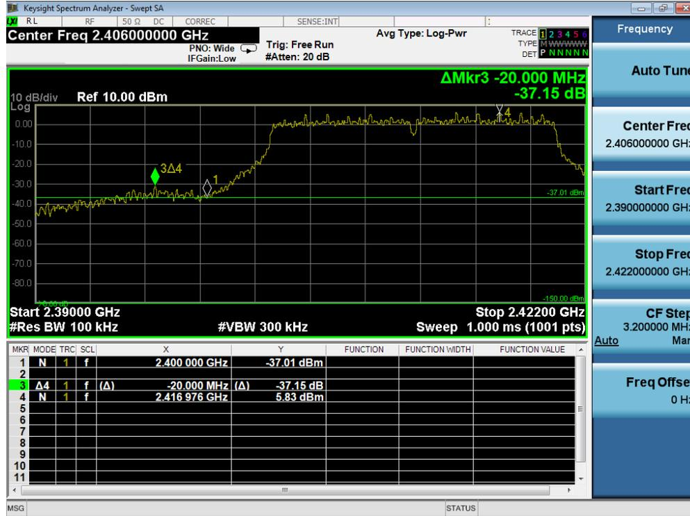
**Conducted Bandedge Average, 2412 MHz, HT/VHT20, M0 to M15**
