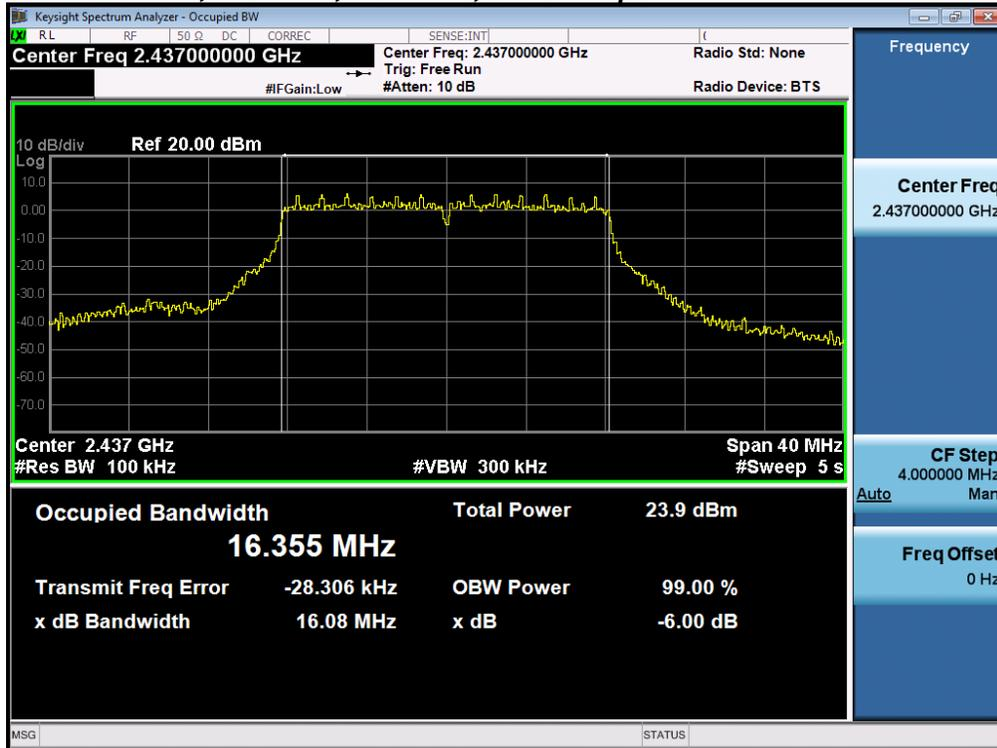
**6dB Bandwidth, 2437 MHz, HT/VHT20, M0 to M15**
