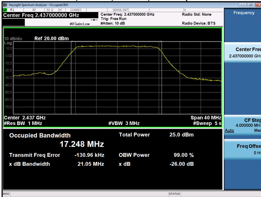
**26dB / 99% Bandwidth, 2437 MHz, HT/VHT20, M0 to M15**
