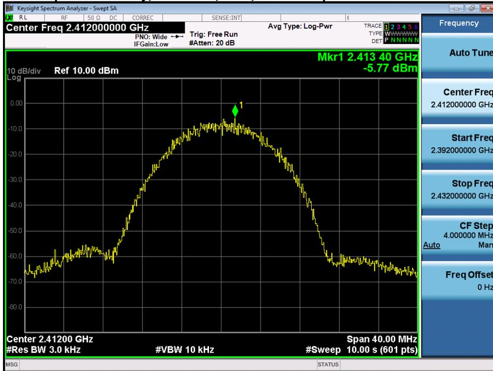
**Power Spectral Density, 2412 MHz, Non HT20, 6 to 54 Mbps**
