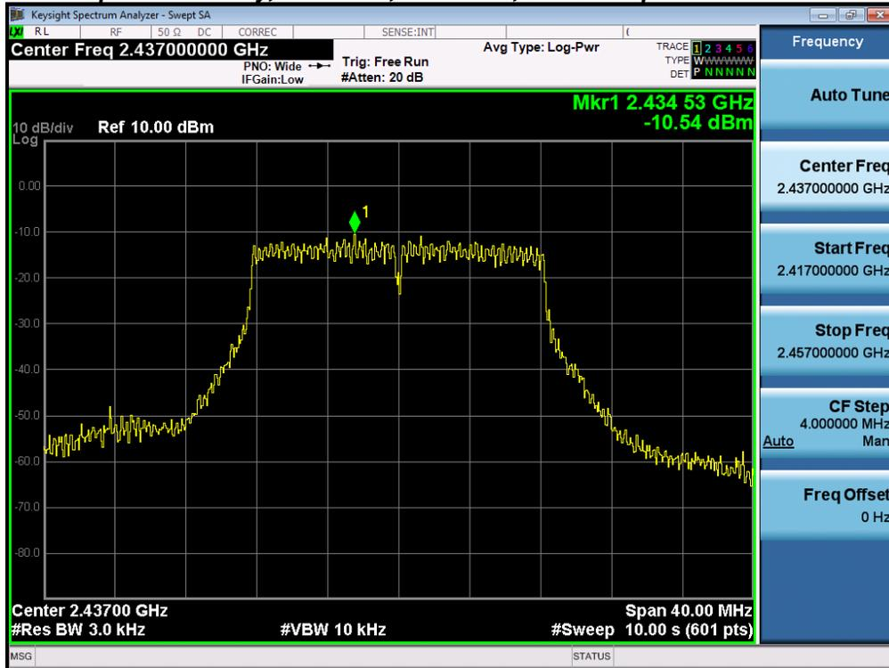
**Power Spectral Density, 2437 MHz, HT/VHT20, M0 to M15**
