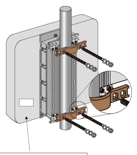
CAUTION: To comply with FCC RF exposure requirements in section 1.1307, a minimum separation distance of 64cm (26 inches) is required between this antenna and all persons.
