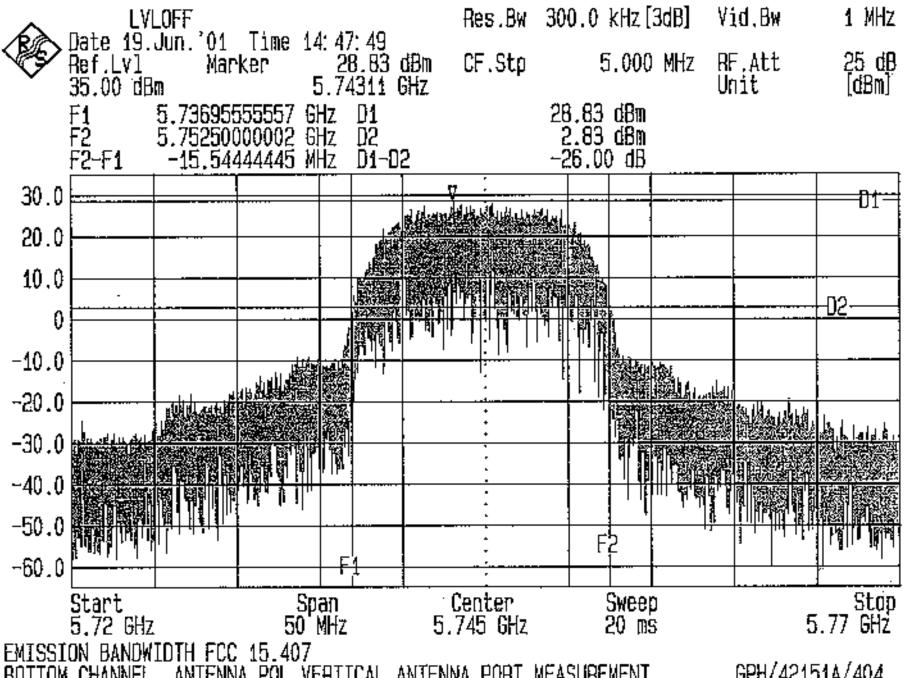
ANTENNA POL VERTICAL ANTENNA PORT MEASUREMENT BOTTOM CHANNEL
