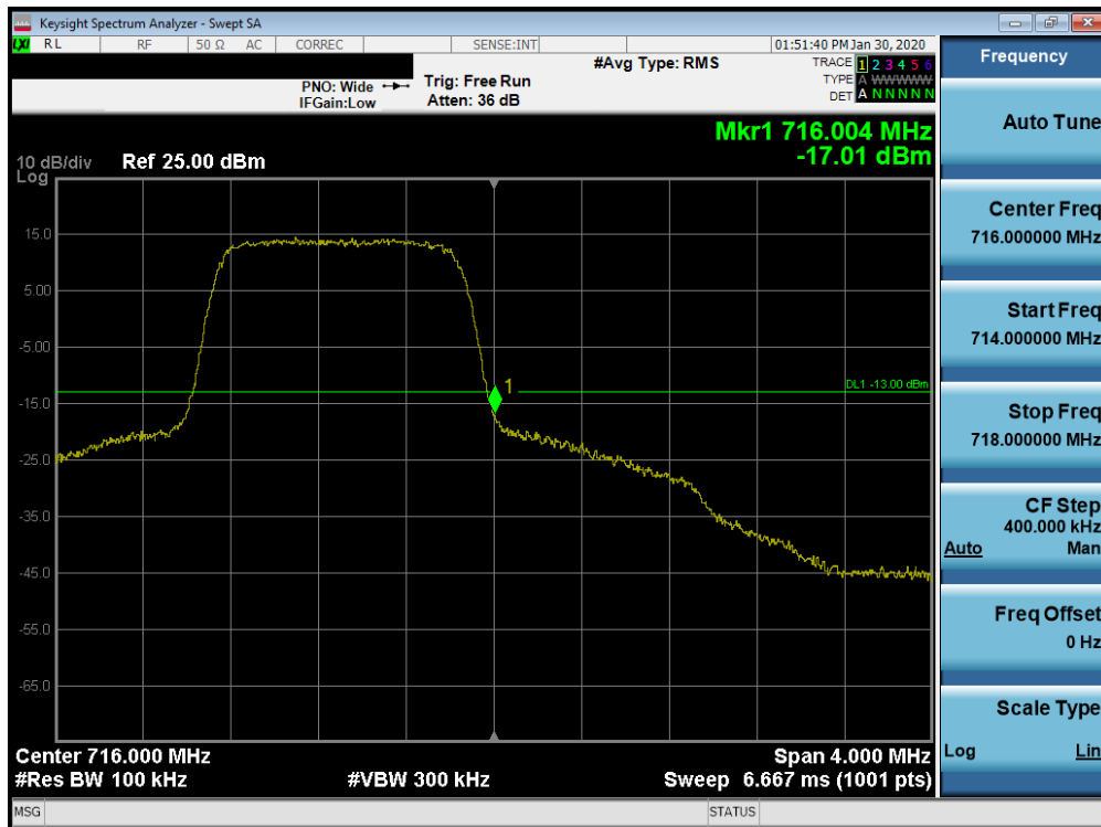
Plot 7-85. Upper Band Edge Plot (Band 12 - 1.4MHz QPSK - Full RB Configuration)
