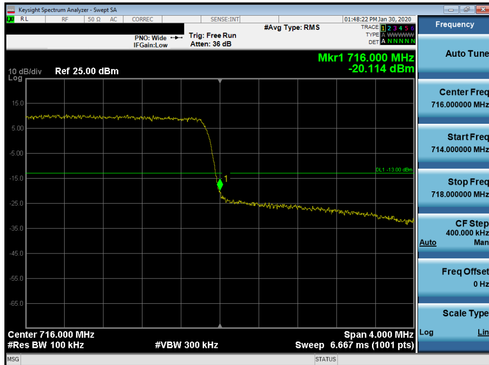
Plot 7-87. Upper Band Edge Plot (Band 12 - 3.0MHz QPSK - Full RB Configuration)
