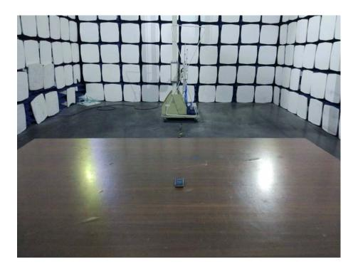
Radiation Emission Test Setup (Above 1GHz)
