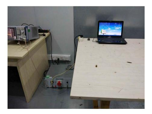
Radiation Emission Test Setup (Below 30MHz)
