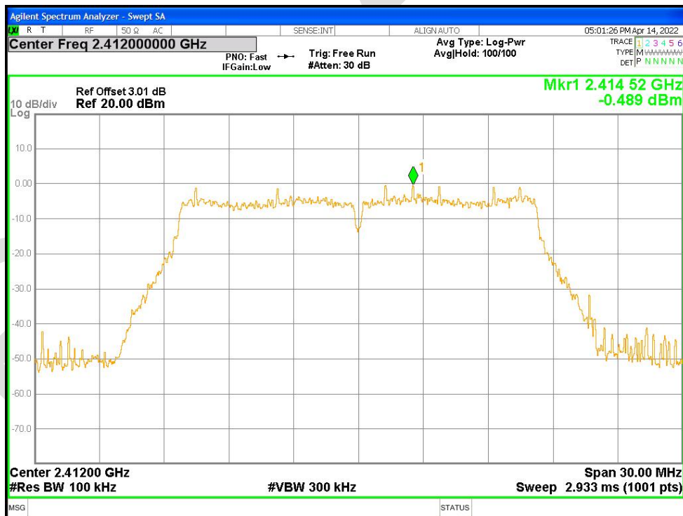
Band Edge NVNT g 2412MHz Ant1 Emission
