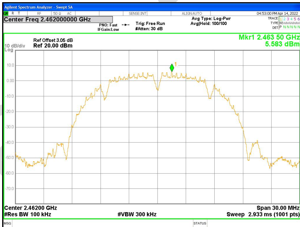
Band Edge NVNT b 2462MHz Ant1 Emission
