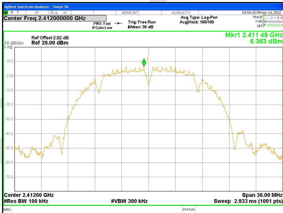
Band Edge NVNT b 2412MHz Ant2 Emission
