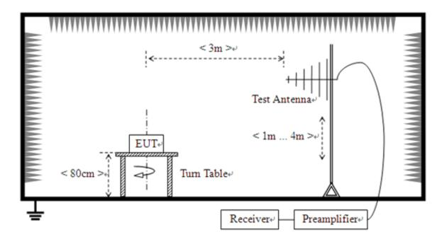
(For Radiated Emission Test (30 MHz-1 GHz))
