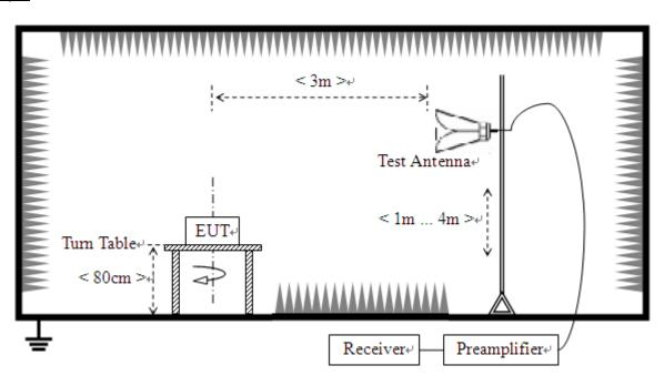
(For Radiated Emission Test (above 1 GHz))
