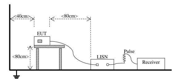
(For Conducted Emission, AC Ports Test)
