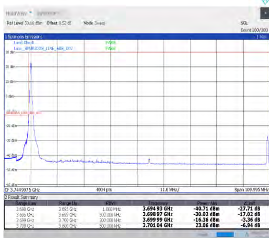
1-N77-3700-3980-30-100-L-4-CP-QPSK-Edge_1RB_L eft-1@0-Ant1-1--PASS-see graph
