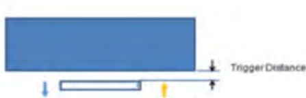
Picture : Proximity Sensor Triggering Distances Assessment (Back/Front Side)
