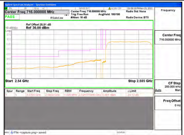
B38 / 15MHz / Low CH / QPSK / FULL RB
