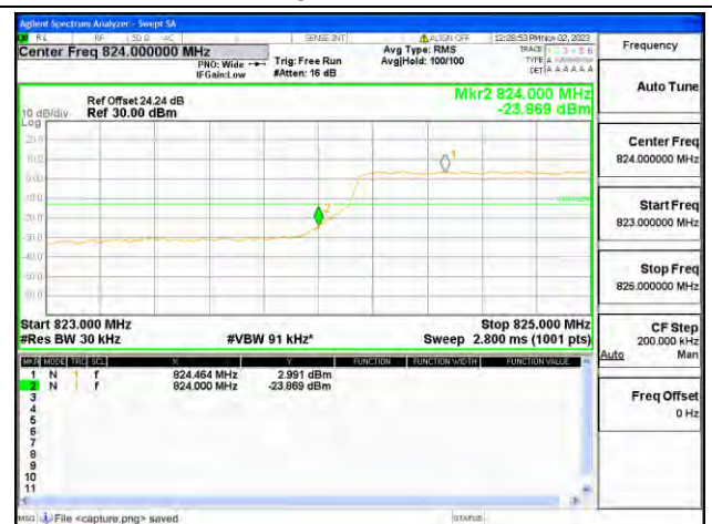
B5 / 3MHz / Low CH / QPSK / FULL RB
