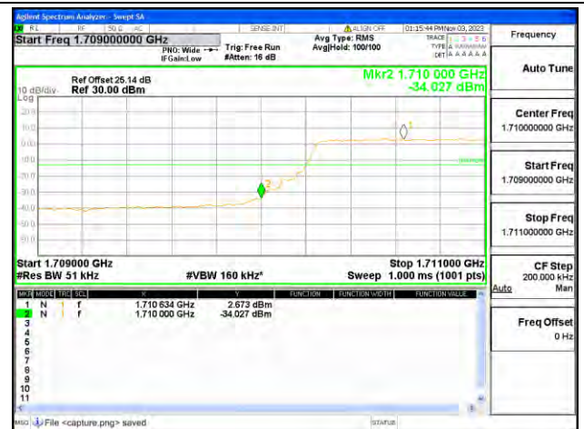
B66 / 5MHz / Low CH / QPSK / FULL RB
