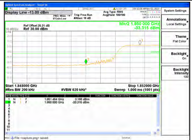
B2 / 20MHz / Low CH / QPSK / FULL RB
