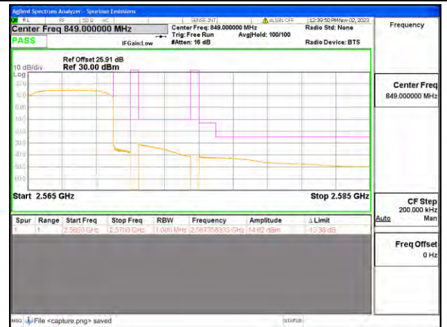
B7 / 5MHz / High CH / QPSK / FULL RB
