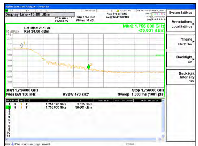
B4 / 15MHz / High CH / QPSK / FULL RB
