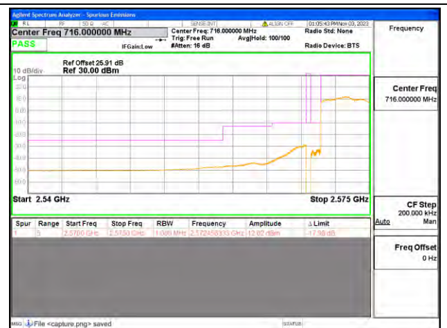
B38 / 5MHz / Low CH / QPSK / FULL RB
