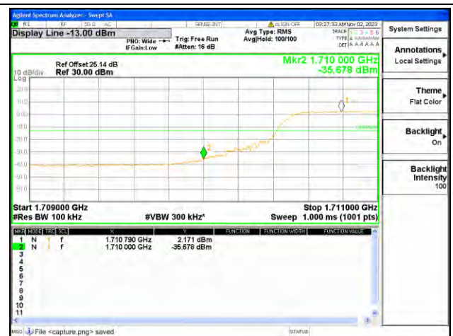
B4 / 10MHz / Low CH / QPSK / FULL RB
