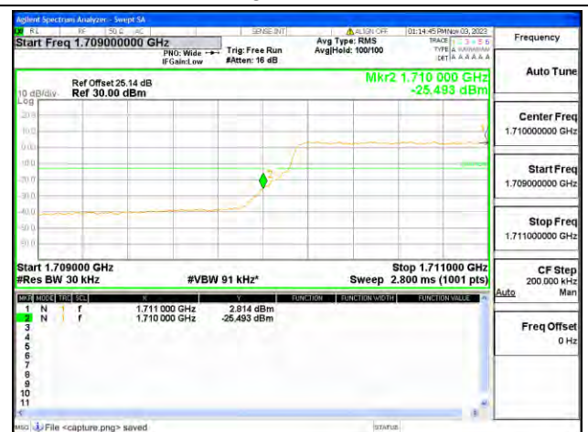
B66 / 3MHz / Low CH / QPSK / FULL RB
