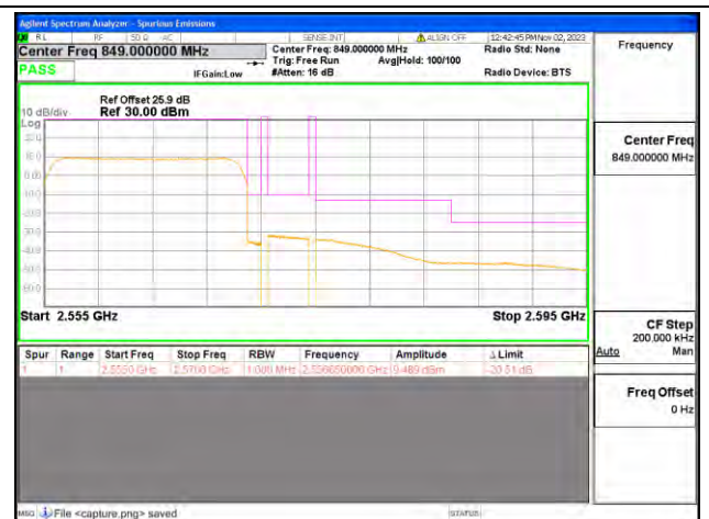
B7 / 15MHz / High CH / QPSK / FULL RB
