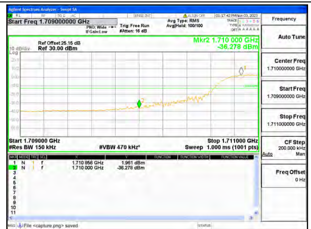
B66 / 15MHz / Low CH / QPSK / FULL RB
