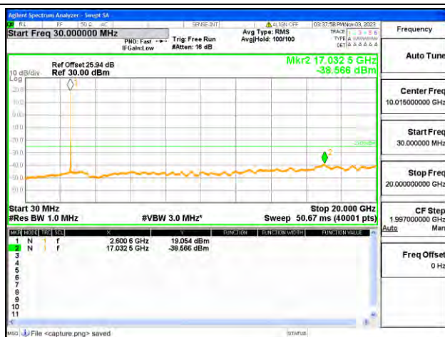
B38-30M-20G / 20MHz / High CH / QPSK
