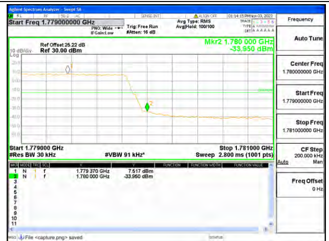
B66 / 1.4MHz / High CH / QPSK / FULL RB
