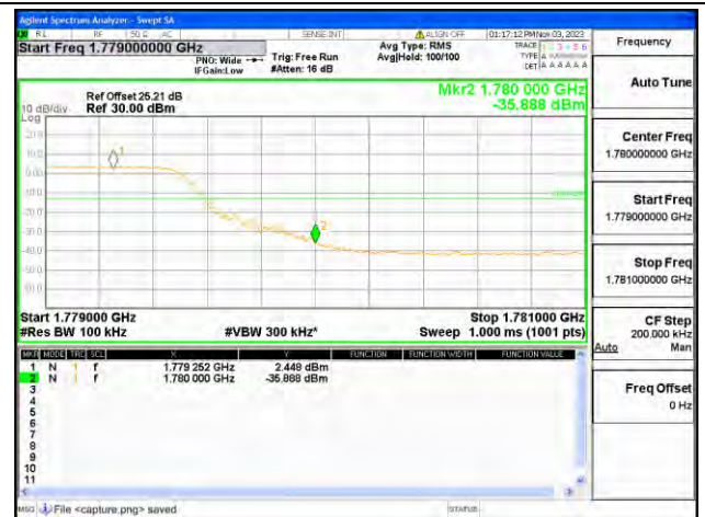
B66 / 10MHz / High CH / QPSK / FULL RB
