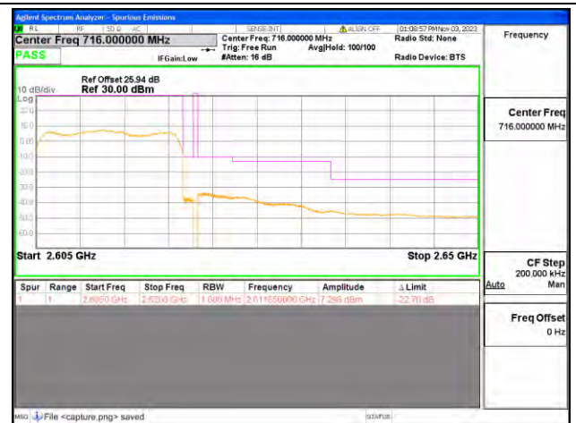
B38 / 15MHz / High CH / QPSK / FULL RB
