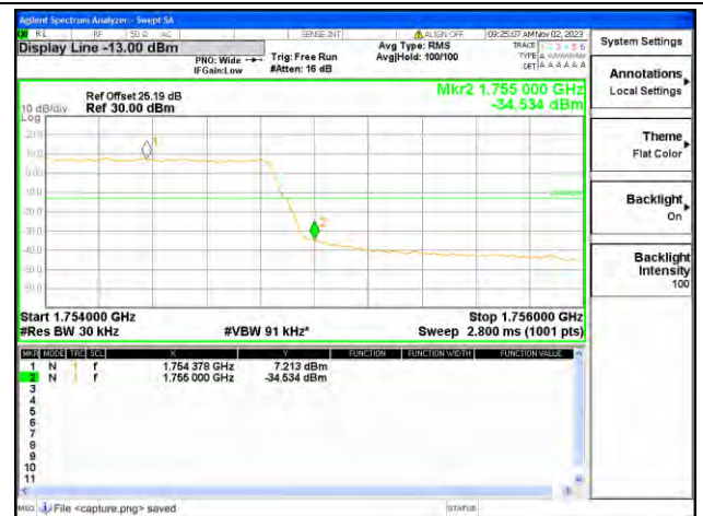
B4 / 1.4MHz / High CH / QPSK / FULL RB
