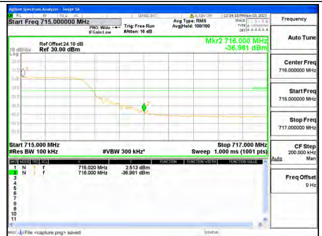
B17 / 10MHz / High CH / QPSK / FULL RB
