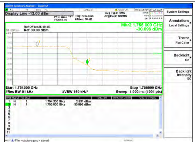
B4 / 5MHz / High CH / QPSK / FULL RB
