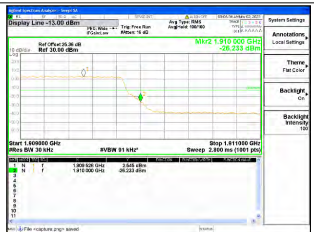
B2 / 3MHz / High CH / QPSK / FULL RB
