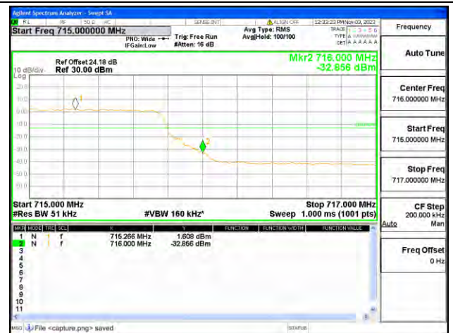
B17 / 5MHz / High CH / QPSK / FULL RB
