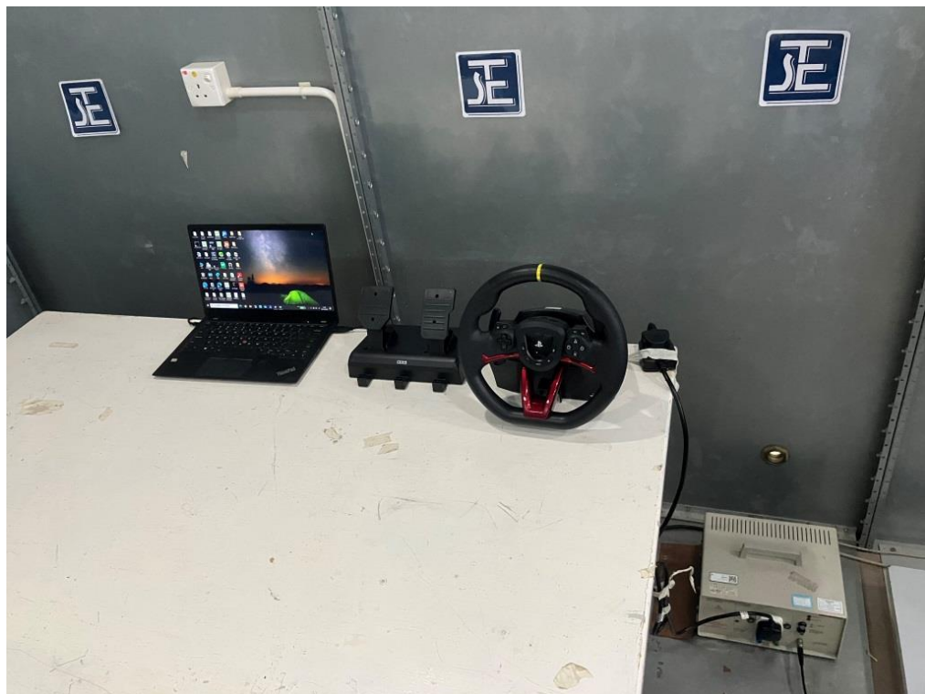
Measurement of Conducted Emission Test Set Up
