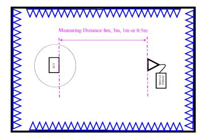
30 MHz - 1 GHz the measuring distance was 3m 1-40 GHz the measuring distance was 4m 40-60 GHz the measuring distance was 3m 60-150 GHz the measuring distance was 1.0m
