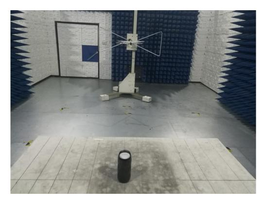
RADIATED EMISSION TEST SETUP ABOVE 1GHZ
