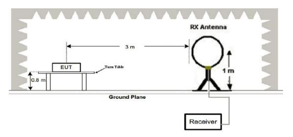
(2) Radiated Emission Test-Up Frequency 30MHz~1GHz
