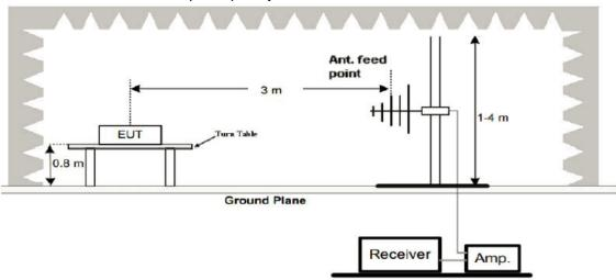
(3) Radiated Emission Test-Up Frequency Above 1GHz
