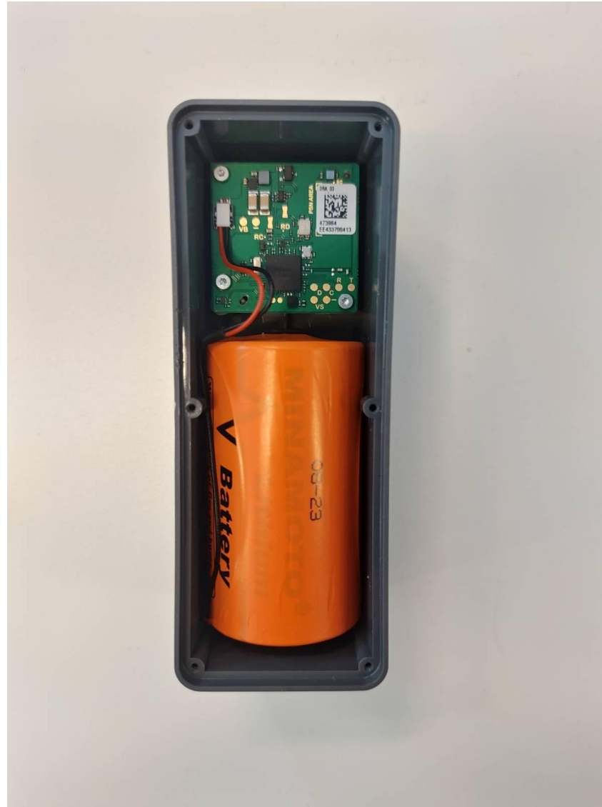
PCB and battery inside A cover
