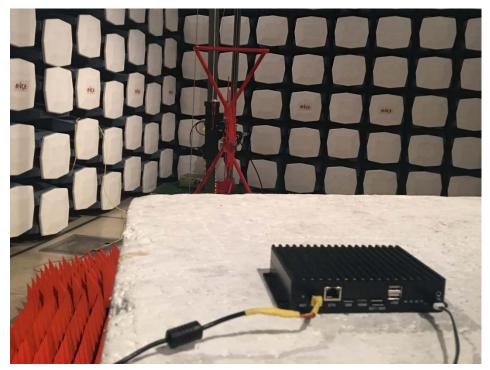
Radiated Emission below 1 GHz Rear View
