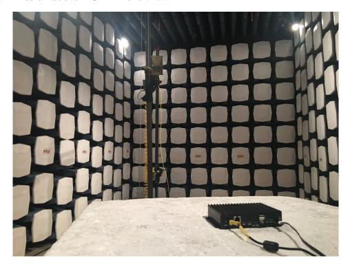
Radiated Emission above 1 GHz Rear View
