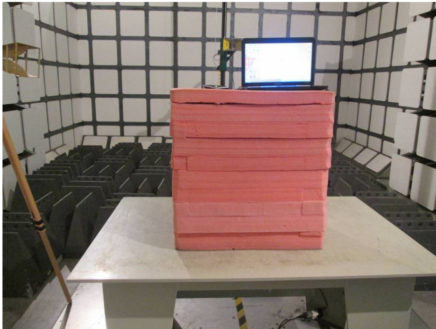
Radiated Emissions View (Above 1 GHz)
