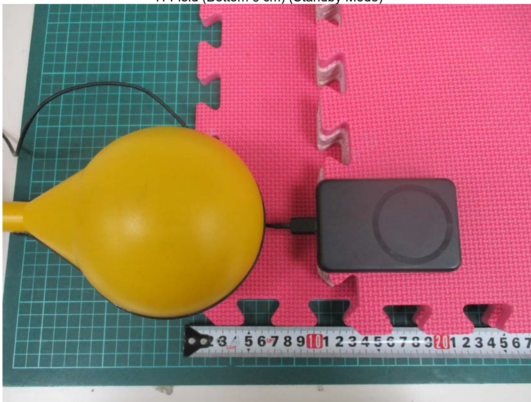
H-Field (Bottom 6 cm) (Standby Mode)
