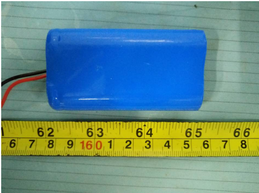
EUT – Battery View
