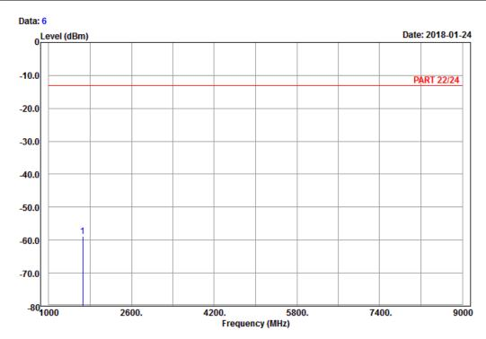
Site : 966 chamber 1 Condition: PART 22/24 Vertical Remark : LTE\_Band 5\_Link\_CH20450
