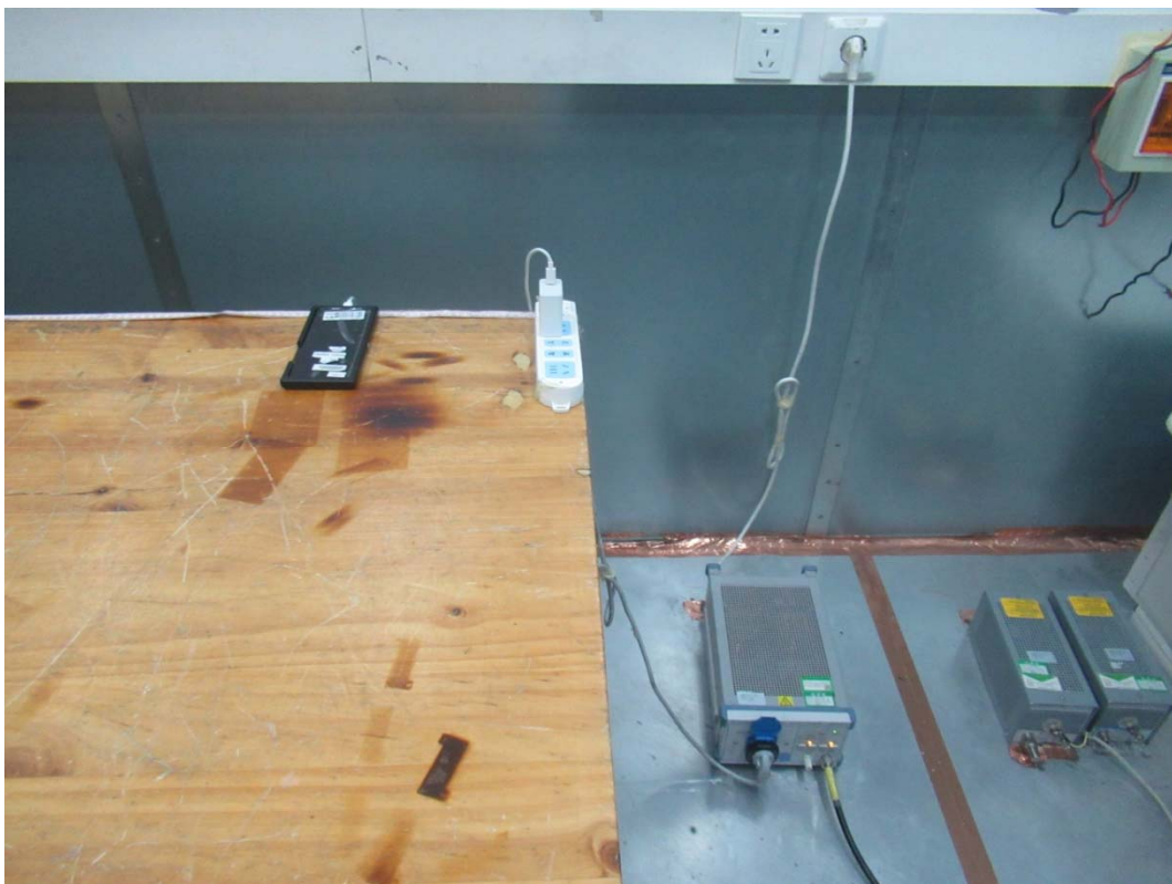
Picture 2 Conducted Emission Test Setup
