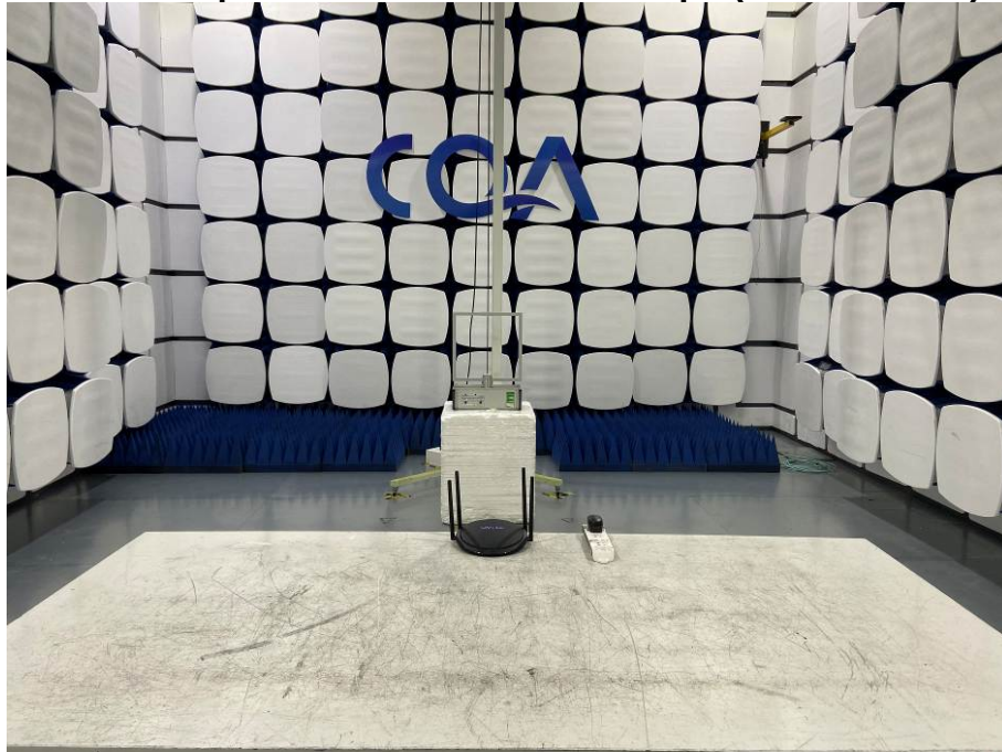
Radiated spurious emission Test Setup-1(Below 30MHz)
