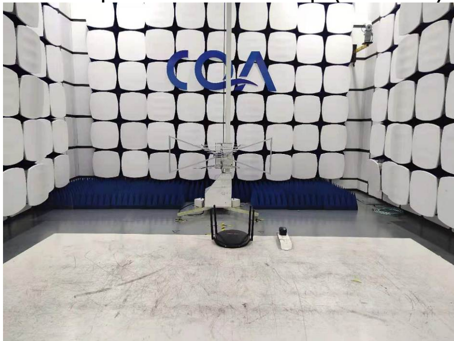
Radiated spurious emission Test Setup-2(30MHz-1GHz)
