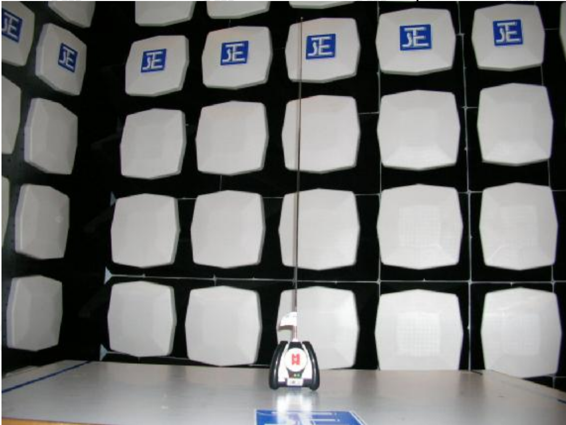
Measurement of Radiated Emission Test Set Up
