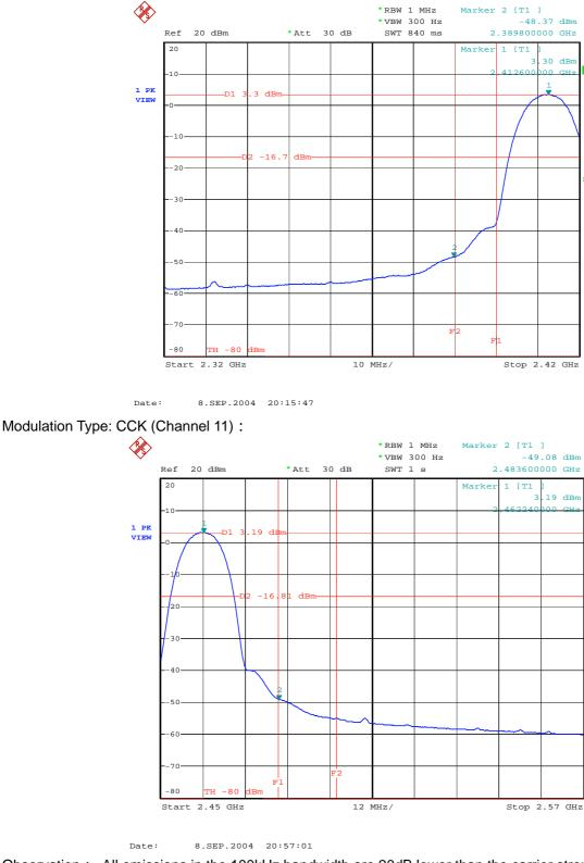
Observation : All emissions in the 100kHz bandwidth are 20dB lower than the carrier strength.
