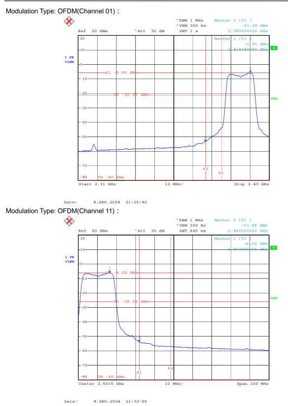
Observation : All emissions in the 100kHz bandwidth are 20dB lower than the carrier strength.
