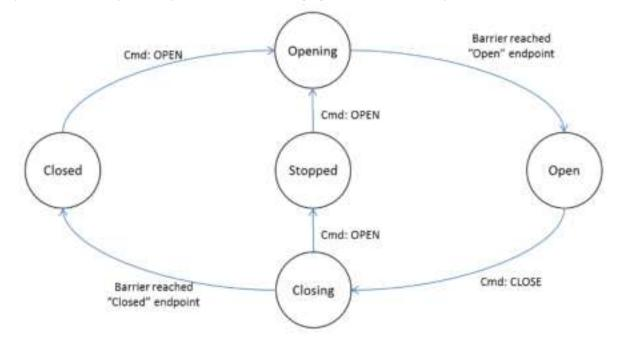
Any state/command pair not specified in the following figure will not cause any action:
