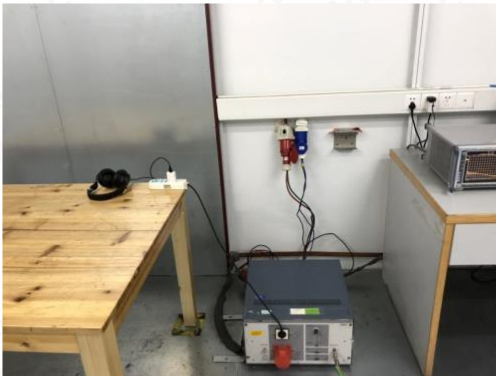
RADIATED EMISSION TEST SETUP BELOW 1GHZ
