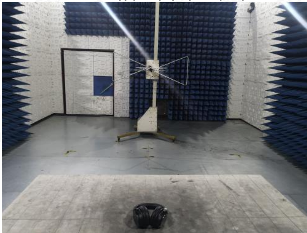
RADIATED EMISSION TEST SETUP BELOW 1GHZ
