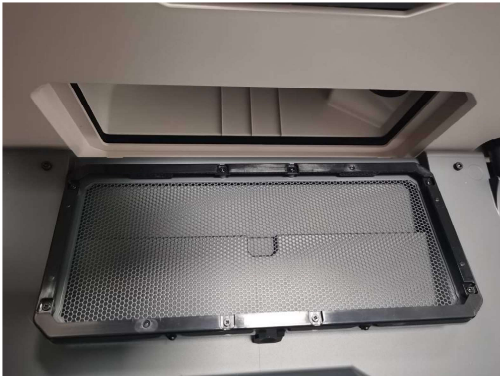
Figure 14. Detachable mesh at venting tunnel
