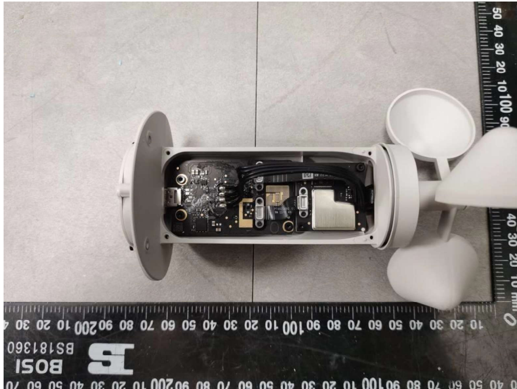
Figure 21. Weather station with potting removed
