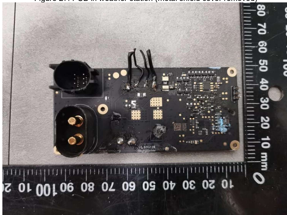
Figure 28. Wireless power transmitter PCB
