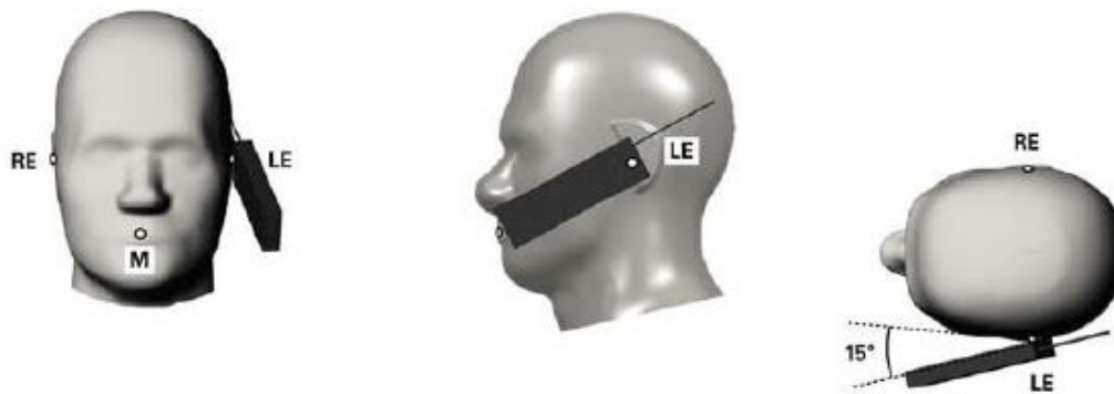
Fig.11.4 Illustration for Tilted Position
