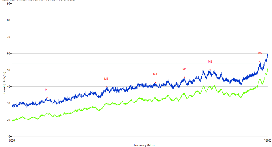
REmission Test case_FCC_Part 15C_FCC 15.247_7GHz-18GHz
