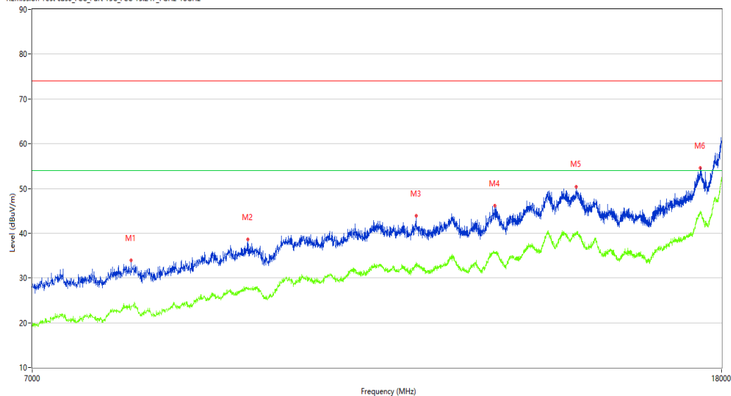
REmission Test case_FCC_Part 15C_FCC 15.247_7GHz-18GHz
