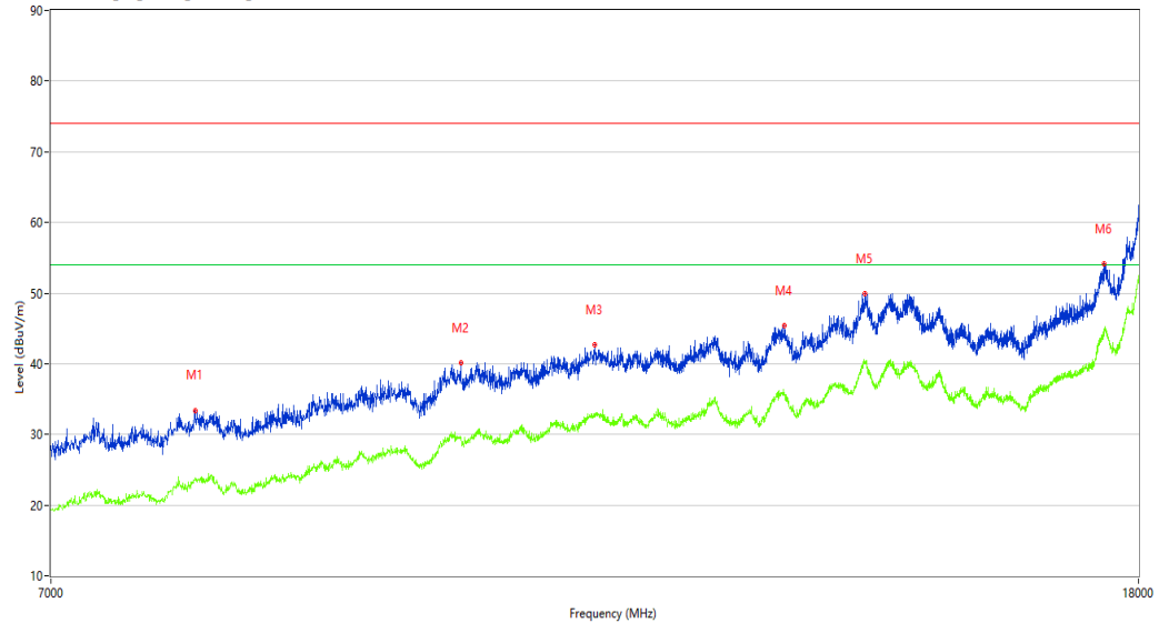
REmission Test case_FCC_Part 15C_FCC 15.247_7GHz-18GHz
