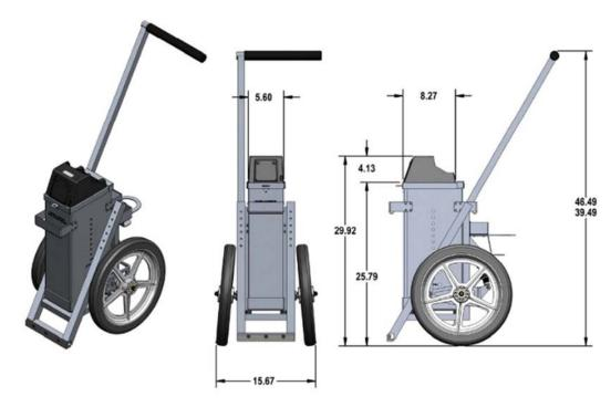
The IPS Collection Cart is a mobile caddy that is used by the city municipalities by the parking meter departments to collect the cash (coins) from the individual street single space parking meters. Each collection cart is equipped with a stainless steel portable collection bucket and the top assembly or upper head assembly has the IPS smart electronics.
