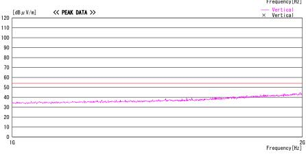
CHART: WITH FACTOR ANT TYPE: -30MHz LOOP, 30-300MHz BICONICAL, 300MHz-1000MHz LOGPERIODIC, 1000MHz-HORN CALCULATION: READING + ANT FACTOR + LOSS (CABLE+ATTEN.) - AMP. GAIN
