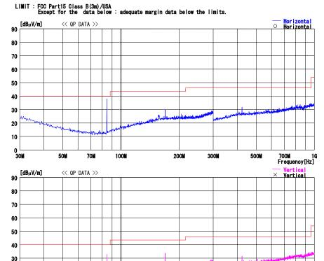
CHART: WITH FACTOR ANT TYPE: -30MHz LOOP, 30-300MHz BICONICAL, 300MHz-1000MHz LOGPERIODIC, 1000MHz- HORN CALCULATION: READING + ANT FACTOR + LOSS (CABLE+ATTEN.) - AMP. GAIN
