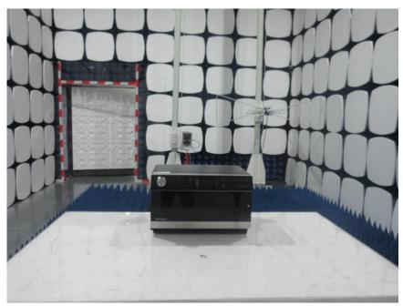
1.4 Operating Frequency Measurement Test Setup
