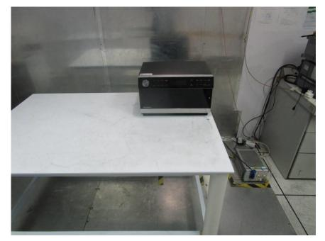
1.2 Radiated Emissions (30MHz-1GHz) Test Setup
