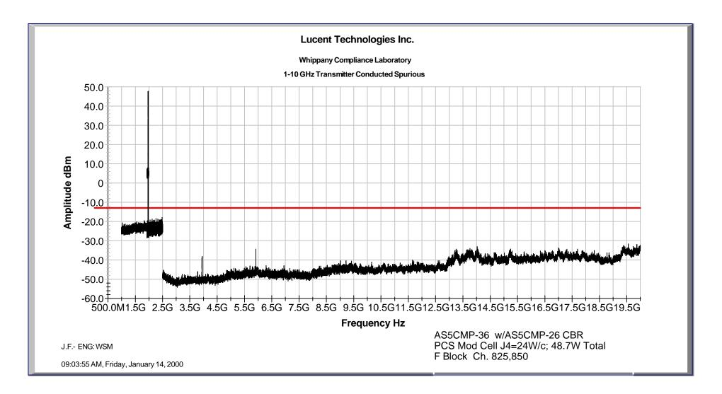
Block F, 3 Carrier Configuration 10 MHz – 10 GHz
