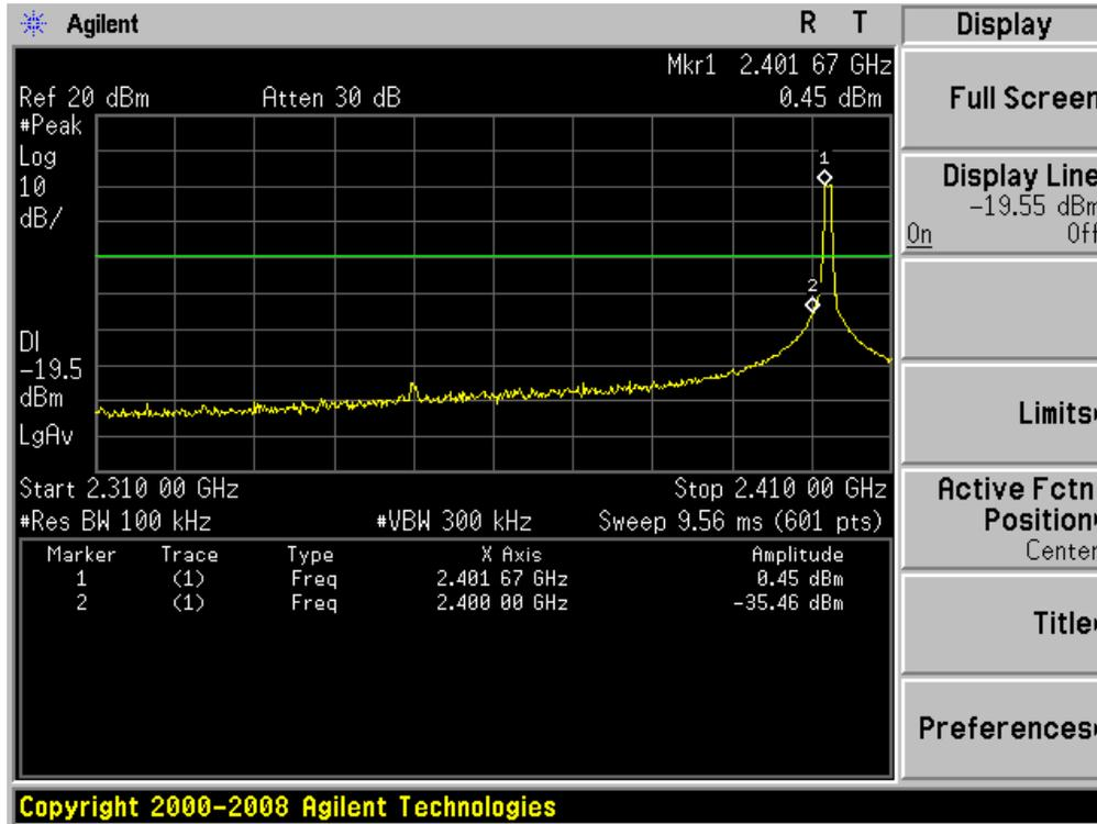
GFSK mode: Band Edge-High Channel
