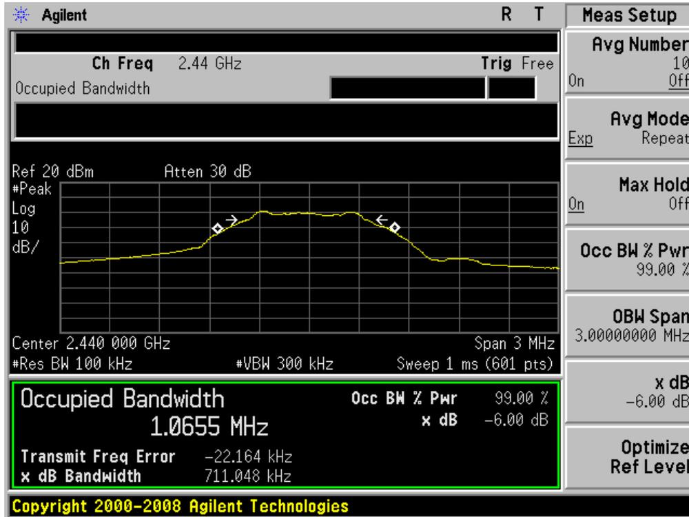
6dB Bandwidth plot on channel 39
