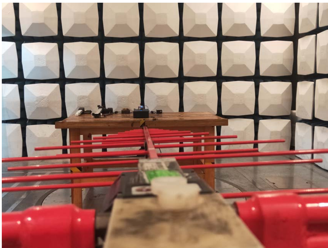
Radiated Emission Above 1GHz View
