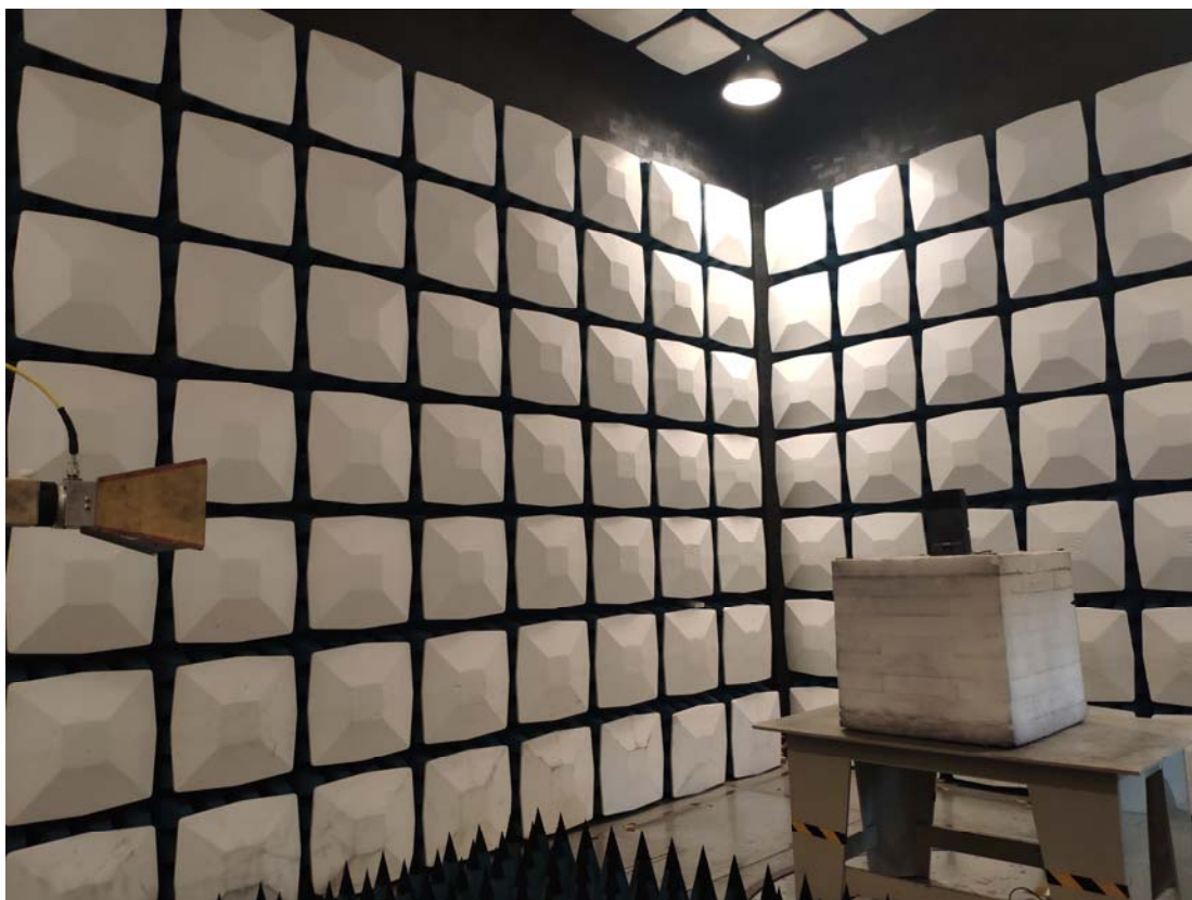
Radiated Emission Above 1GHz View
