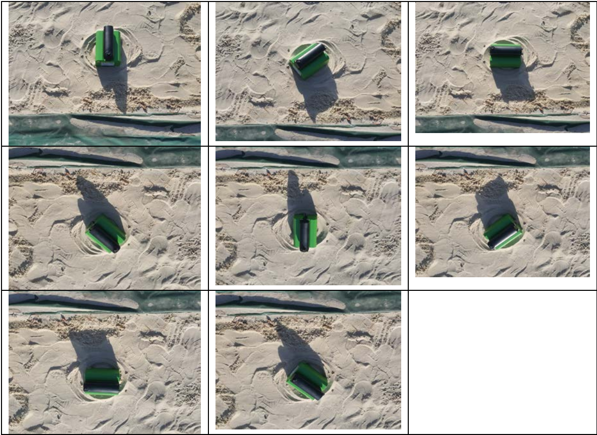
EUT Positions with 45 Degree Interval
